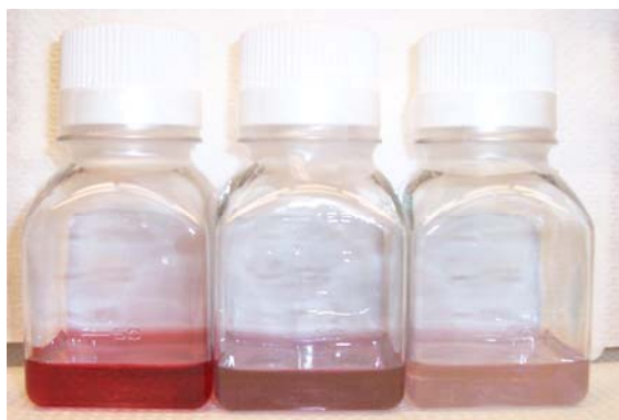
Figure 5: Gold Nanoparticles of different sizes. As gold nanoparticles increase in size they change from red to blue (from left, 30 nm, 60 nm, and 90 nm gold nanoparticles.)
