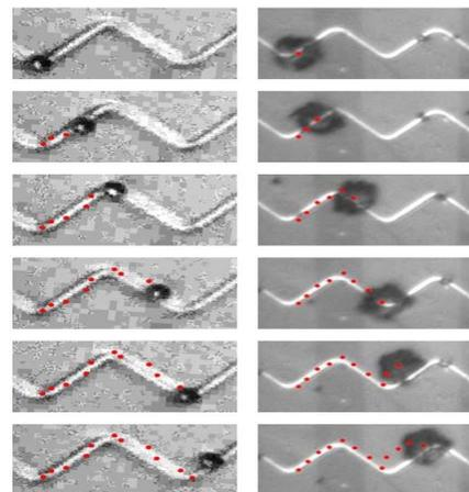
Transport (*a la* joystick) of a micro sphere (left) and T-lymphocyte cell (right) on a Si platform along a zigzag wire. Trajectories indicated by red dots.
